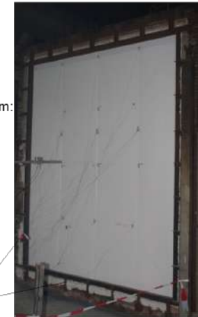
Sandwich panel façade test
